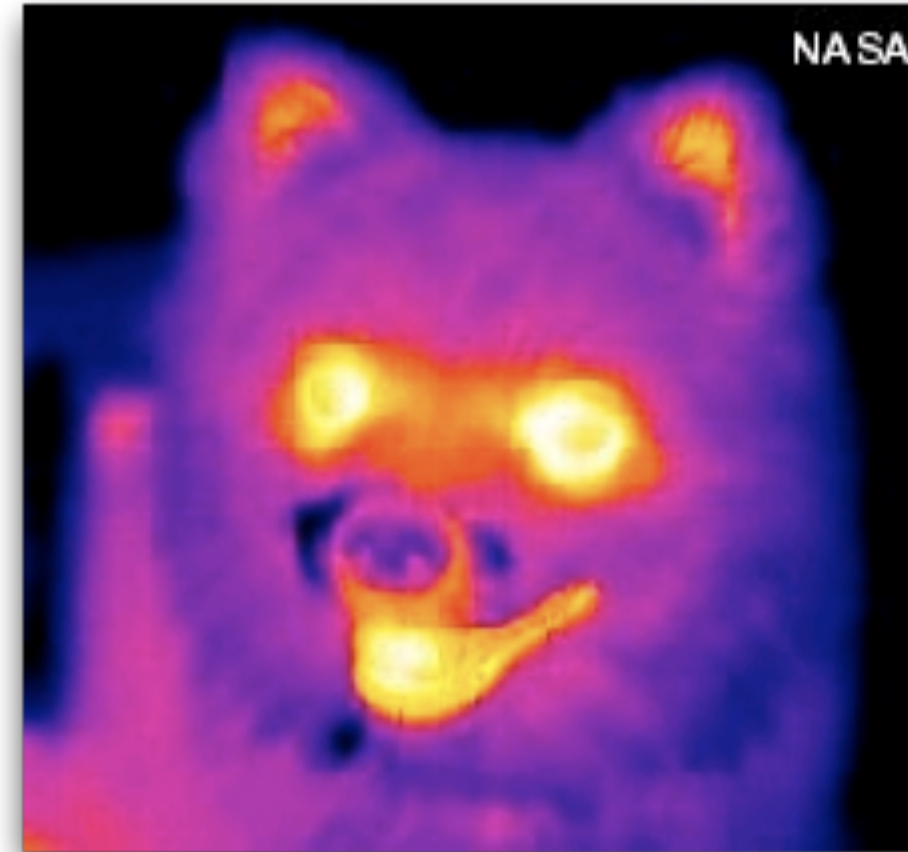
Infrared photograph of a dog shows warm temperatures as yellow or white.
